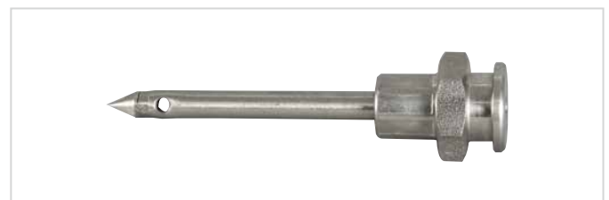
Figure 15: Joint injection needle (No. 23207), Ø 5 mm x 71 mm, stainless steel, lateral outlet openings Ø 2.5 mm; working length 25 mm, connection pan head nipple with check-valve, AF17
