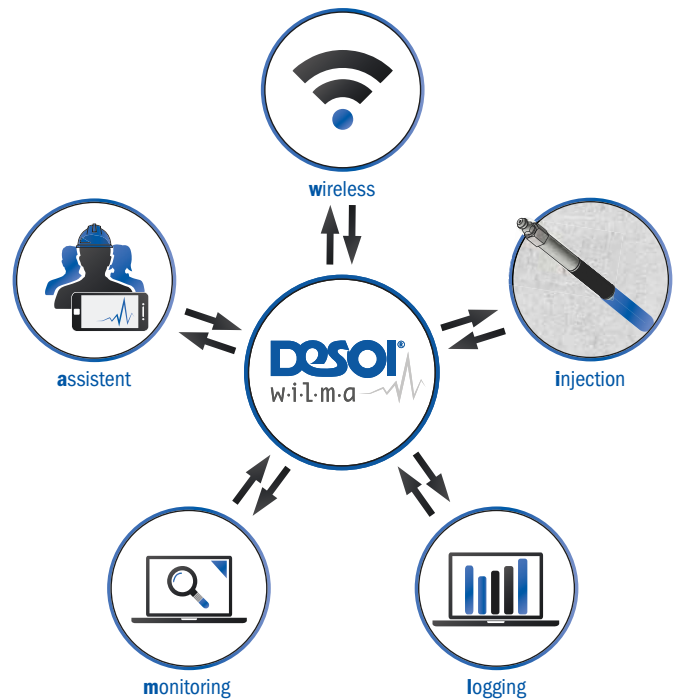
Figure 31: Basic representation of the functions of the data logger w.i.l.m.a.
