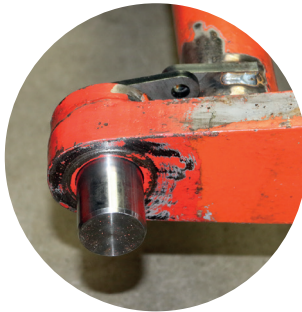
⑤ Lower bearing with additional anti-rotation protection of the bolt
