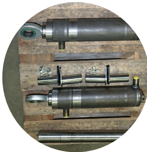
⑧ New hydraulic cylinder set with centre shear bolt and bearing bolt
