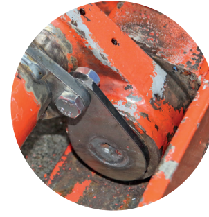
② Lower running rail inside the platform, running rail with wear strip on the running surface
