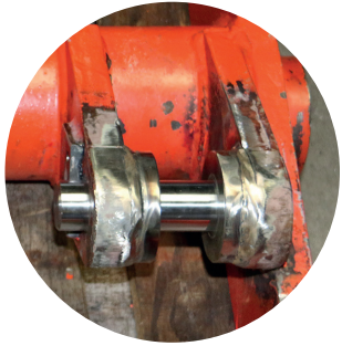
① Cylinder suspension renewed on both sides at the top of the inner shear
