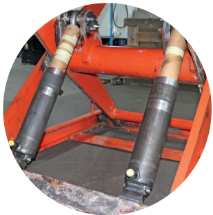
⑦ View into the inside of the scissor lift (cylinder side) after the overhaul
