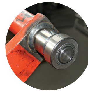
⑨ Upper roller with new and reinforced bearing journal
