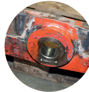
⑥ Renewed bearing for the middle shear bolt
